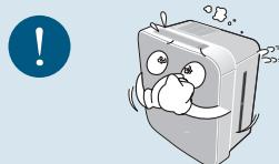
**Don't drain water remaining in the water tank by holding body frame and drain water by eliminating water tank.**
